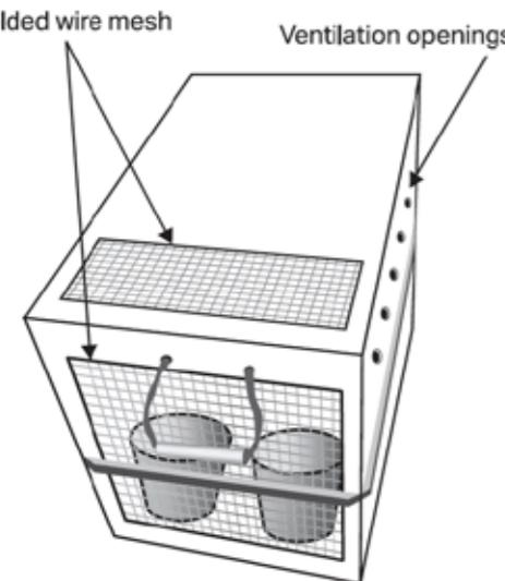
Ventilation must be provided on all 4 sides of the container. Ventilation openings on the sides and the back must be placed over the upper two thirds of the container.
